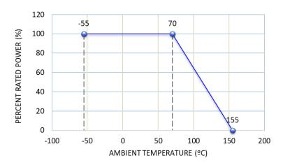
Power rating or current rating is in the case based on continuous full-load at ambient temperature of 70°C. For operation at ambient temperature in excess of 70°C, the load should be derated in accordance with figure of derating curve.
