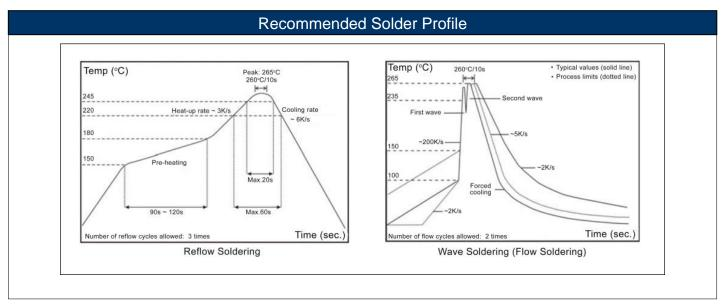
Rework temperature (hot air equipment): 350°C, 3~5 seconds Recommended reflow methods: IR, vpor phase oven, hot air oven
