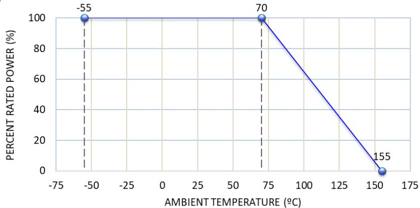
Power rating or current rating is in the case based on continuous full-load at ambient temperature of 70°C. For operation at ambient temperature in excess of 70°C, the load should be derated in accordance with figure of derating curve.
