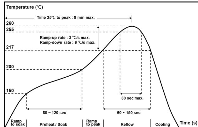
Rework temperature (hot air equipment): 350°C, 3 ~ 5 seconds
